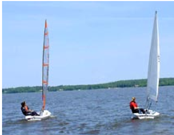
Note the closed leech on the standard Byte on the right. In the light conditions pictured, there is nothing the sailor can do to open that leech - and it is slow.
